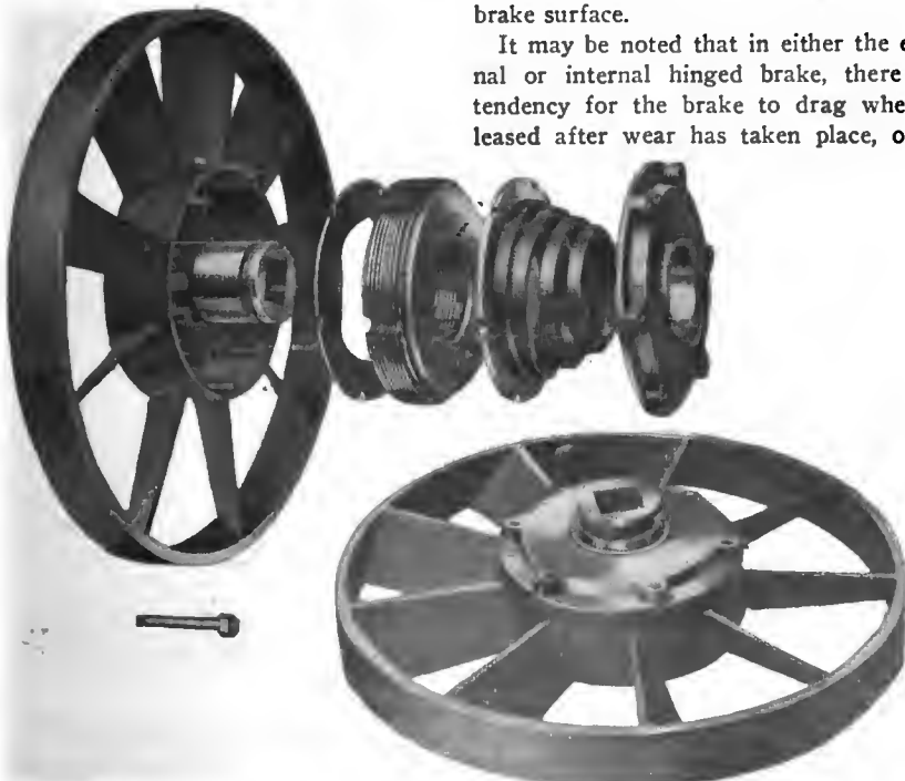
VIEWS OF FRANKLIN MULTIPLE DISK CLUTCH ASSEMBLED AND APART.
